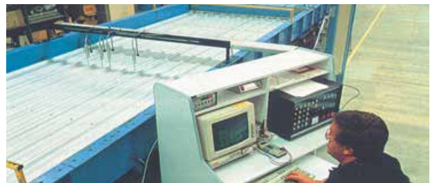
Wind Pressure Testing Rig
