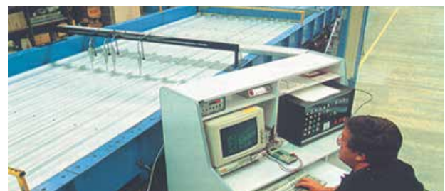
Wind Pressure Testing Rig
